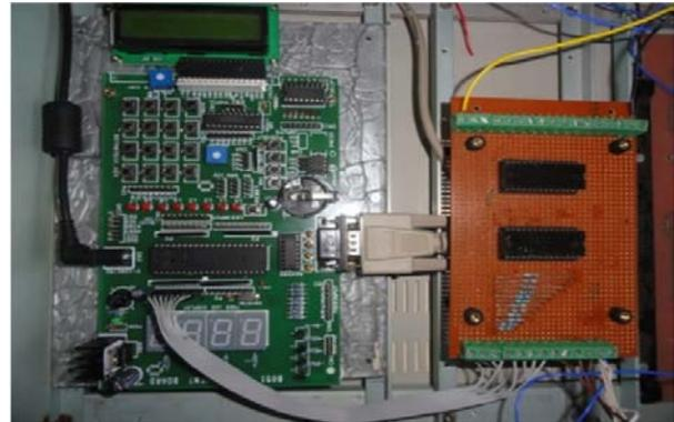
**Fig. 5: Prototype of the ASCS. Right side board consists of the resistor bank, analog multiplexer ICs and the terminal blocks for interfacing. The left side board is the 8051 microcontroller based development kit (P89V51RD2).**
